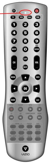
NOTE: This is a programmable remote supporting up to 4 devices (see TV, VCR, CABLE, DVD buttons at the top of the remote). If the remote is not working with your VIZIO TV, press the TV button on the remote to set the functions back to TV.
